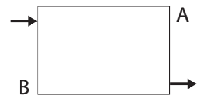
TBOE top-bottom opposite end, side, left hand flow
